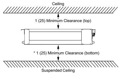
\* NOTE - Bottom unit clearance can be 1 inch (25 mm), but allow 12 inches for filter removal on end return air applications
