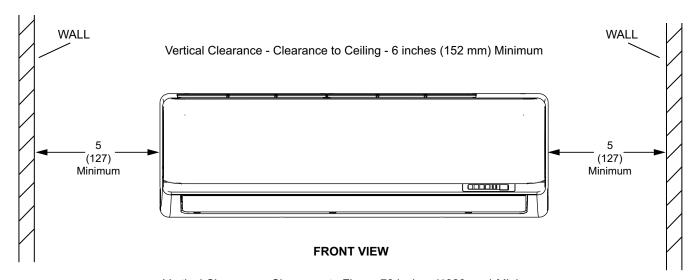
Vertical Clearance - Clearance to Floor - 72 inches (1829 mm) Minimum NOTE - Provide 96 inches (2438) clearance to floor for best performance
